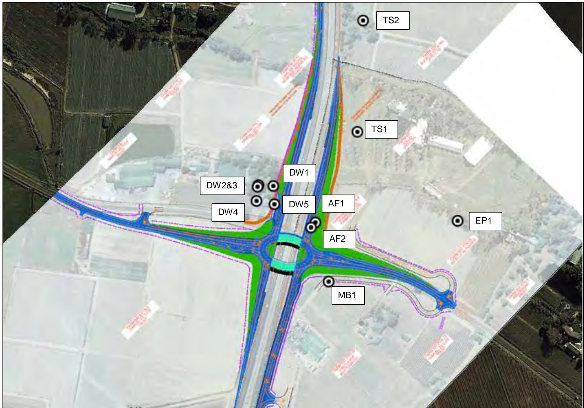
Figure 6.8: Position of boreholes at the intersection of the R44 with Annandale Road in relation to the proposed grade-separated roundabout
