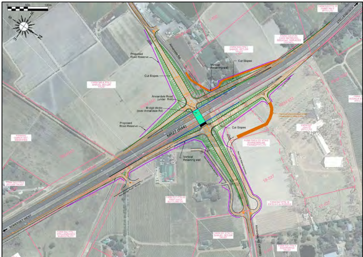
Figure 4.14: Proposed below-ground grade-separated diamond interchange at the Annandale Road Intersection with fill slopes (K&T, 2015)
