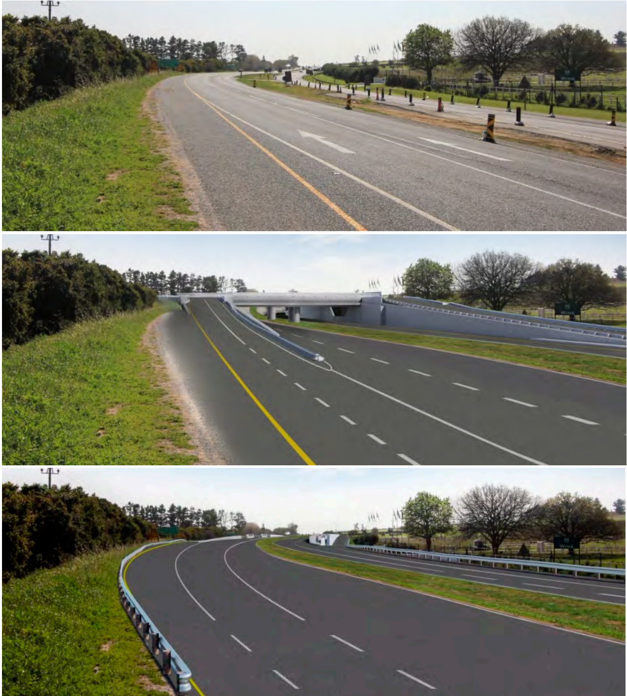
Figure 6.2: Visual simulations of proposed grade-separated alternatives at the R44/Winery Road Intersection, showing the view looking north – composite image comparing an existing view (top image ) with photomontages of the proposed above-ground roundabout (middle image) and the proposed below-ground interchange (bottom image) (Think3dlab, 2016).
