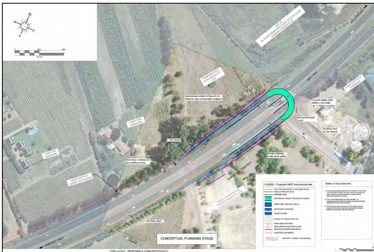
Figure 4.15: Proposed grade-separated U-turn facility near Jamestown Cemetery (K&T, 2015)
