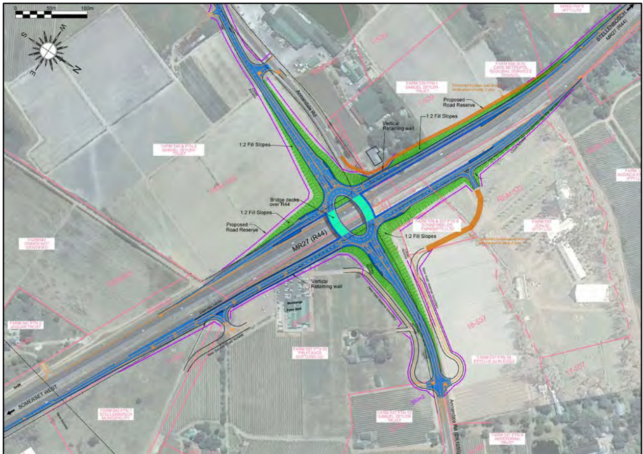
Figure 4.12: Proposed grade-separated roundabout at the Annandale Road Intersection with ramp embankments (K&T, 2015)
