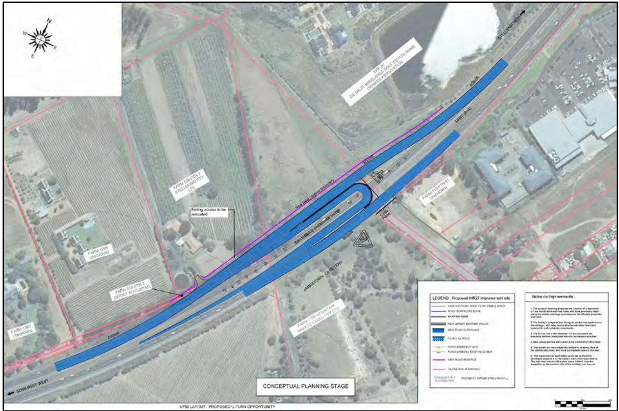
Figure 4.16: Proposed at-grade U-turn facility near Jamestown Cemetery (K&T, 2015)
