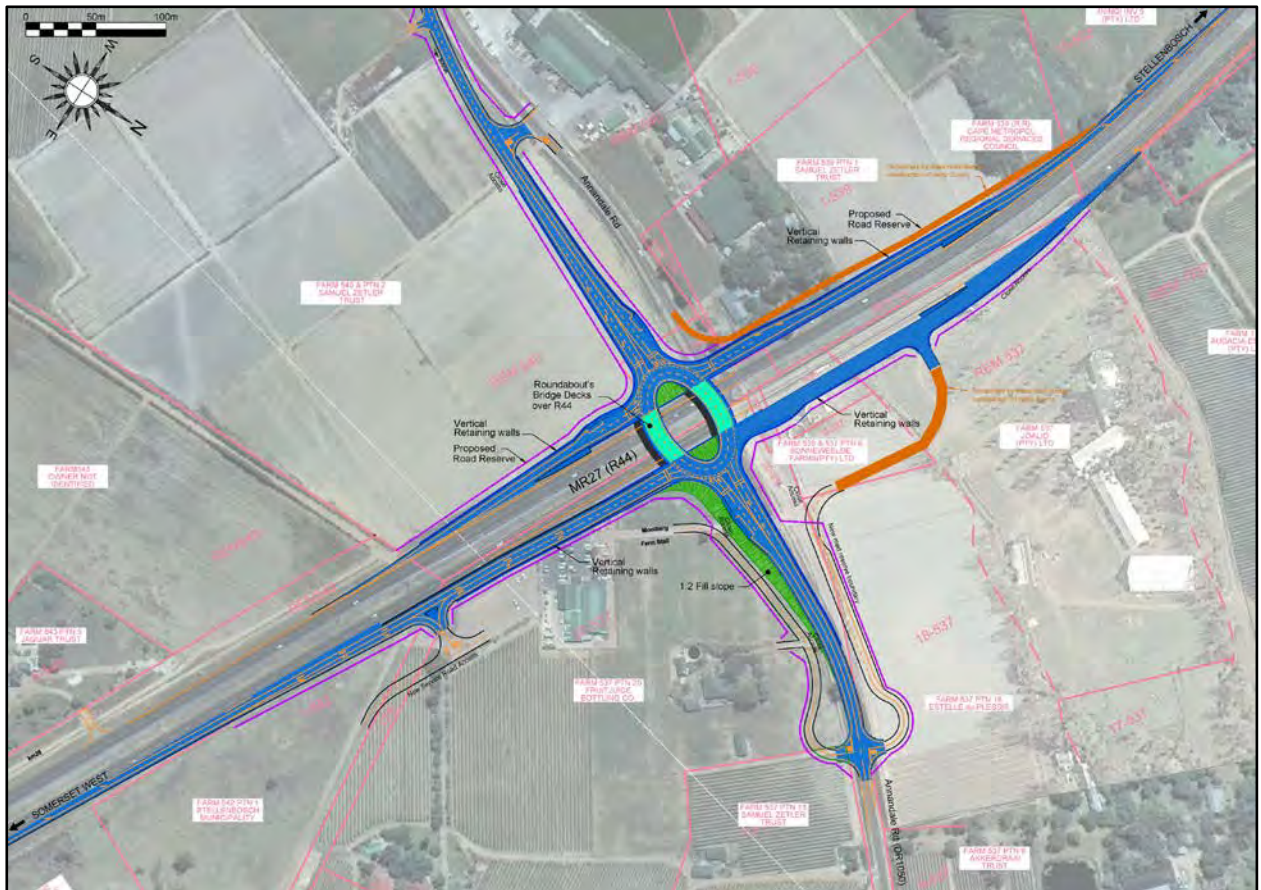
Figure 4.13: Proposed grade-separated roundabout at the Annandale Road Intersection with vertical retaining walls (K&T, September 2015)
