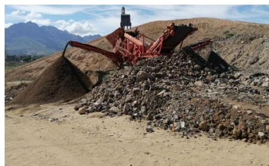
Figure 18: Crushing of builder's rubble done on site
